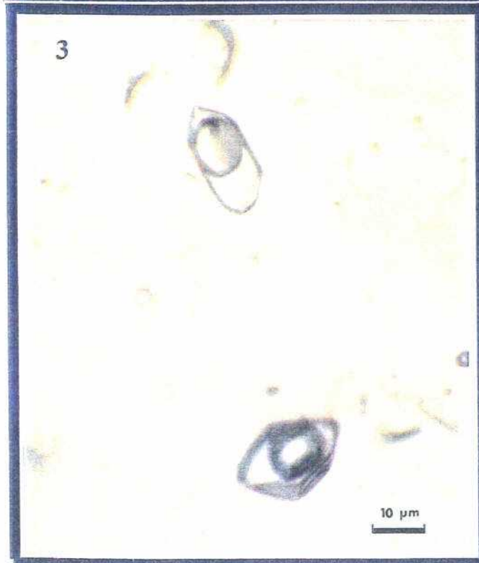
Plate IV-15 : Fluid inclusion features from Penedono area (Dacotim and St Antonio Mine);
